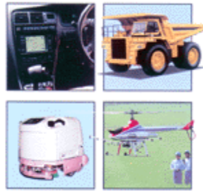
Fig. 6.6. Hitachi FOG for Toyota dashboard display (upper left), cleaning robot (lower left), and autonomous dump truck and helicopter applications (right). Describing the automotive application, an Hitachi brochure states, "The FOG detects rotation of cars...allowing you to know the direction in which you are headed....and travel to the desired destination in a minimum amount of time." The Hitachi brochure also describes the important role such systems would play in intelligent vehicle highway systems.
